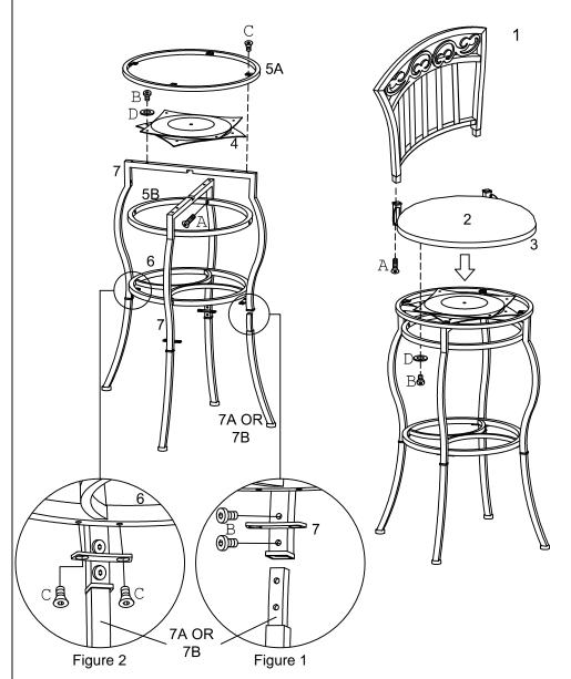
Step 1. Insert four Extension Legs (7A or 7B) into the legs 7 as shown (If you want a counter stool use 7A, for bar stool height use 7B). Attach the extension legs by inserting (8) allen bolts B into each hole. See Figure 1. Tighten all (8) bolts B at this time
