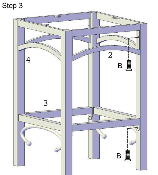
Step 1: Attach Top Stretcher [2] to Leg Assembly [4] by inserting (1) Allen Bolt [B] into hole as shown. Repeat for other Top Stretcher [2].
